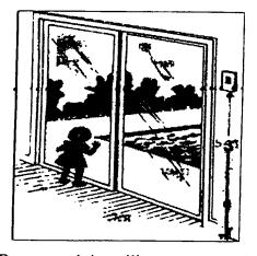
1) All doors which give direct access to a swimming pool must be equipped with an audible alarm which sounds when the door and/or screen are opened. The alarm must sound for 30 seconds or more immediately after the door is opened. The alarm must be capable of being heard throughout the house during normal household activity. (The alarm sound should be distinct from other sounds in the house, such as the telephone, doorbell and smoke alarm.) The alarm must have an automatic reset feature.
