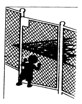
These are the gates people must walk through. Swimming pool barriers should be equipped with a gate or gates which restrict access to the pool. A locking device must be included in the gate design. Pedestrian gates must open outward and away from the pool and shall be self-closing and self-latching.
