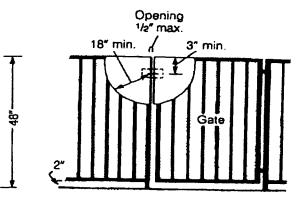
The release mechanism shall be located at 54" or higher from the bottom of the gate.
